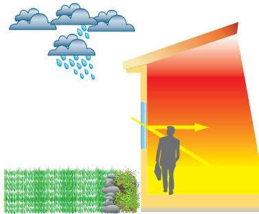
**U-Value ( $U_w$ )** measures how readily a window conducts heat. It is a measure of the rate of non-solar heat loss or gain through the assembly. The rate of heat is indicated in the terms of the U-Value of a window assembly which includes the effect of the frame, glass, seals and any spacers. The lower the U-Value, the greater a window's resistance to heat flow and the better its insulating value.
