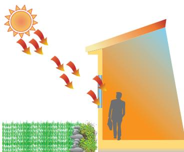
**Solar Heat Gain Coefficient (SHGC<sub>w</sub>)** measures how readily heat caused by sunlight flows through a window. The SHGC<sub>w</sub> is the fraction of incident solar radiation admitted through a window, both directly transmitted, and absorbed and subsequently released inward.
