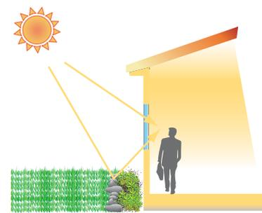
**Visible transmittance ( $T_{vw}$ )** measures how much light comes in through a window. It is an optical property that indicates the amount of visible light transmitted.
